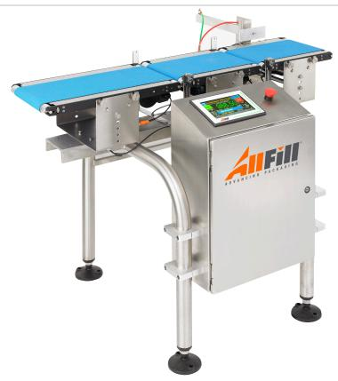
The Model EW-8 is All-Fill's economical solution for users and applications that may only require an entry level checkweigher. The EW-8 offers 0.5g resolution. It utilizes a strain gauge load cell for weighing packages up to 5 lbs and operating at speeds up to 120 packages per minute, this makes the EW-8 just as versatile and reliable as other All-Fill models.
